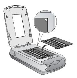
Note: If you're scanning 35-mm slides, set the holder on the scanner first, then place the slides in the holder.
